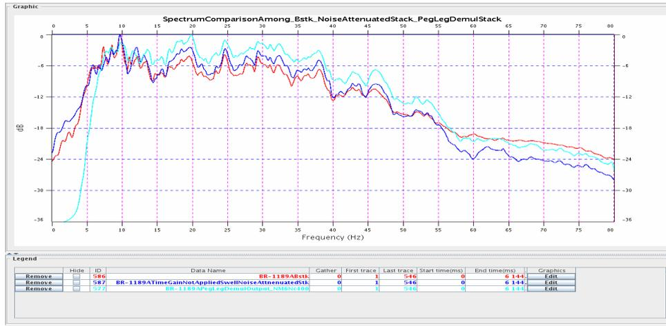
Figure 6. Amplitude spectra for raw (in red), noise attenuated (in violet) & peg-leg removed (in blue) stack
