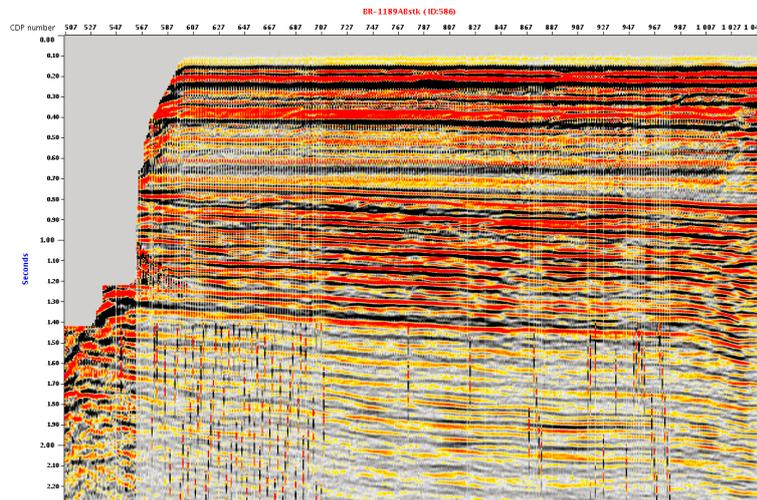
Figure 2. Raw stack without noise attenuation
