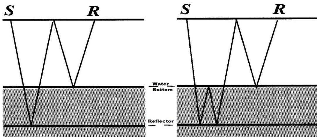
**Figure. 1** Raypaths associated with first & second order peg-leg multiples, where S corresponds to air-gun source & R to hydrophone receiver
