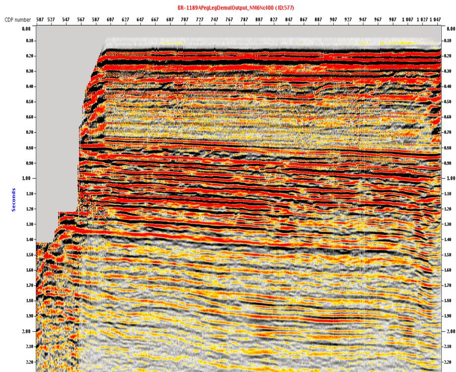
Figure 5. Peg-leg attenuated stack
